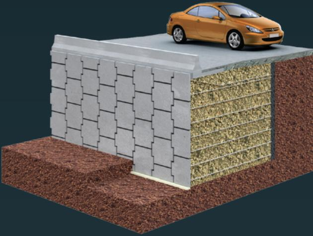
The original Reinforced Earth® technique combines select granular, engineered backfill with steel or synthetic tensile reinforcements and a modular facing system. This ideal combination creates a durable, mass gravity retaining wall.
